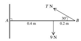
A non-uniform rod AB, of length 0.6 m and weight 9 N, has its centre of mass 0.4 m from A. The end A of the rod is in contact with a rough vertical wall. The rod is held in equilibrium, perpendicular to the wall, by means of a light string attached to B. The string is inclined at  $30^{\circ}$  to the horizontal. The tension in the string is T N (see diagram).
